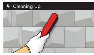
Once the stones are firmly affixed, clean the surface with a dry brush to clear the stones of any dust
