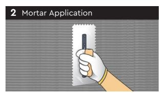
Apply a generous layer of mortar across the wall using the notched edge of a trowel, creating a "combed" surface pattern.
