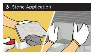
• Complete this step starting from the bottom of the wall & moving upwards: Apply a thick layer of mortar onto the back side of stone. Press and hold the stone firmly onto the mortared wall surface for a few seconds. Repeat this until the section is completed with stones. Use spacers and leveler if necessary to ensure a level arrangement.
